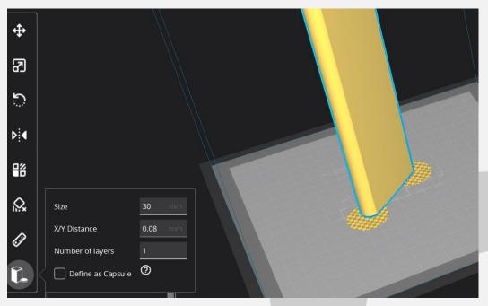
Once completed, be careful when removing these tabs from the print as they are quite strong and can damage the bottom of your part if not removed carefully. Re-open any holes the tab may have filled on the bottom of the print.
