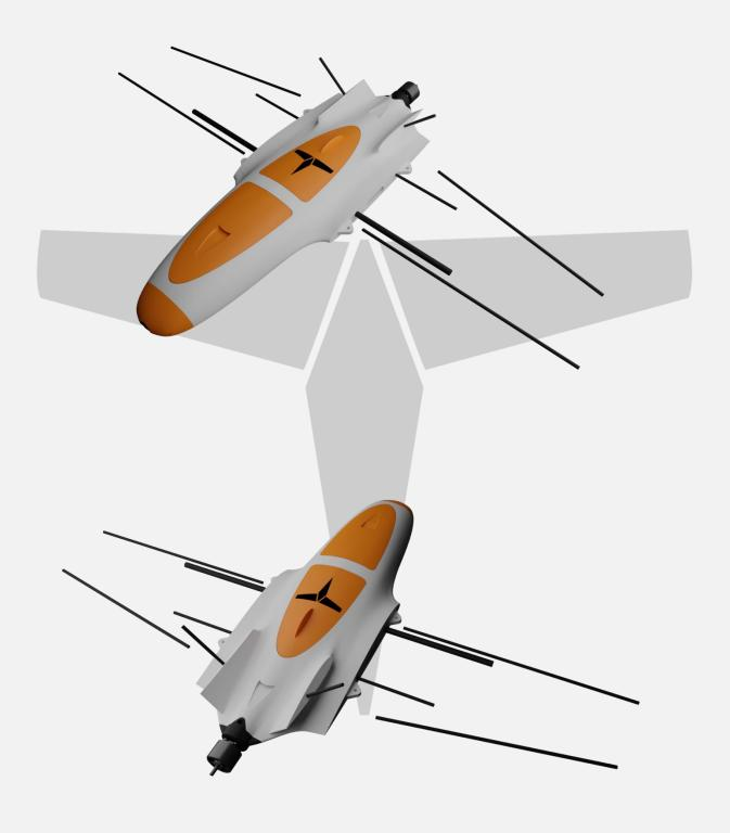
• Medium CA glue should be used to assemble all fuselage parts.
