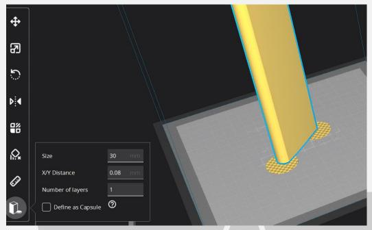
Once completed, be careful when removing these tabs from the print as they are quite strong and can damage the bottom of your part if not removed carefully. Re-open any holes the tab may have filled on the bottom of the print.
