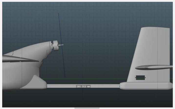
Please make sure the tail boom's exposed length is ~200mm. Feel free to adjust based on CG or desired stability (farther away = more stable, closer = more acrobatic). Stay within +- 20mm of the recommended distance.
