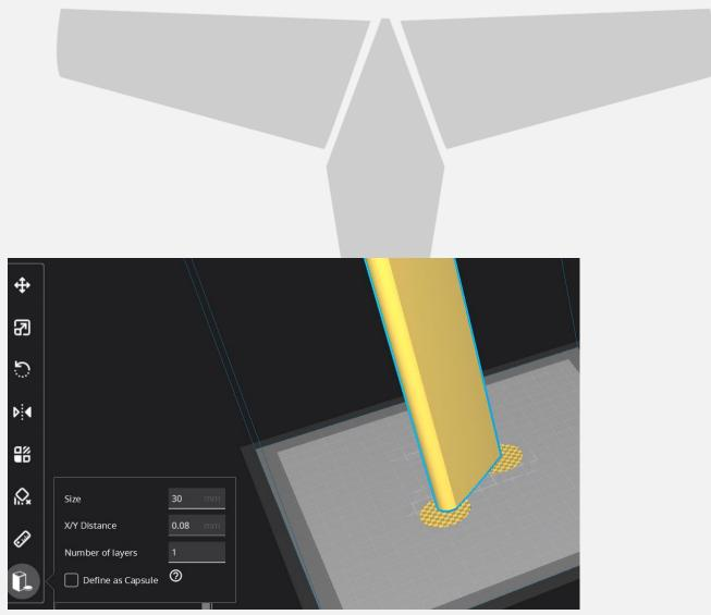
Once completed, be careful when removing these tabs from the print as they are quite strong and can damage the bottom of your part if not removed carefully. Re-open any holes the tab may have filled on the bottom of the print.
