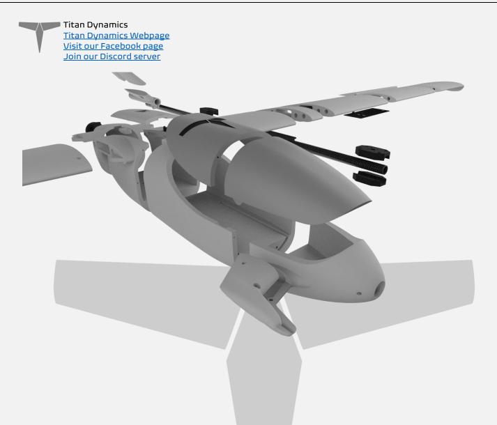
The spar layout for Cobra is as depicted below. None of the spars need to be glued in, they will all be retained by the printed parts. The two wing spars that intersect the fuselage are the joiners for the wings and the fuselage and can be removed completely from the fuselage and wing during transport. The booms can also be removed, as well as the tail
